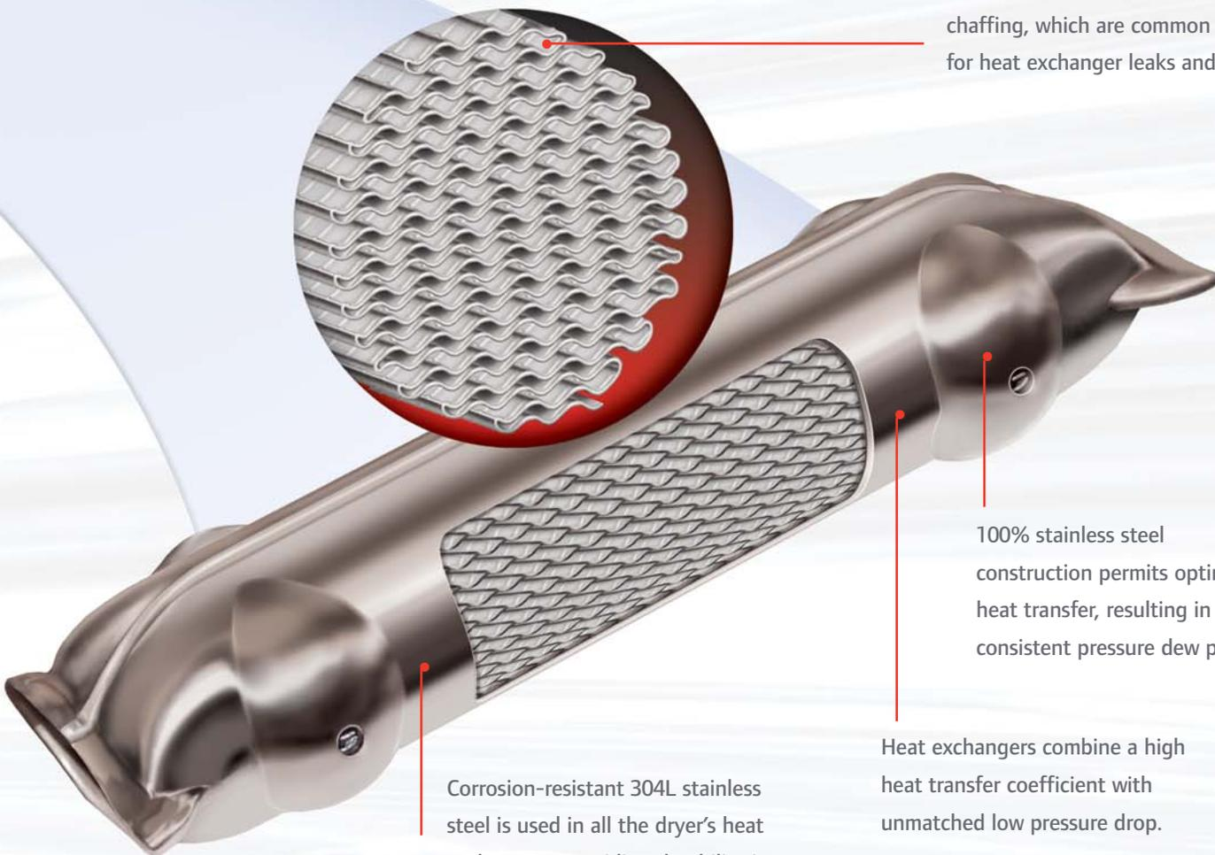
Corrosion-resistant 304L stainless steel is used in all the dryer's heat exchangers, providing durability in environments unsuitable for copper or other metals.
